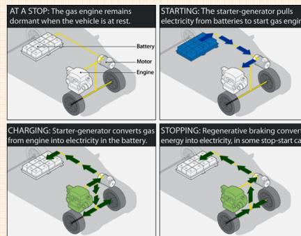
Start-Stop system uses **regenerative braking** when you want to apply brake when engine is on. The rotational energy from wheels turns the electric generator and creates electricity. The generator sends electricity to the
